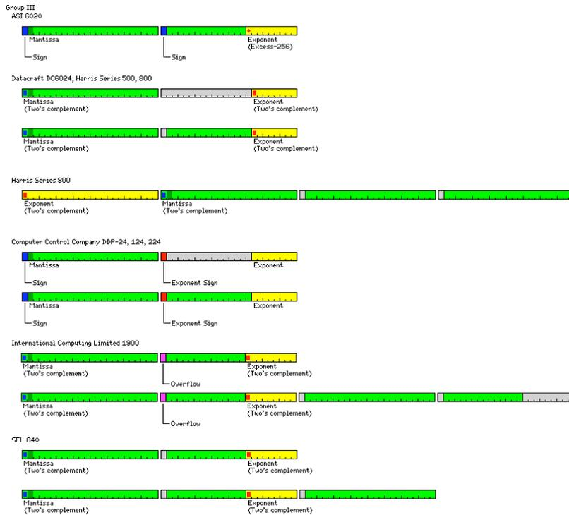
The ASI 6020 computer used a 39-bit mantissa in sign-magnitude format, followed by a nine-bit exponent in excess-256 notation, a rare instance of excess-n format being used in a Group III representation of floating-point numbers.
