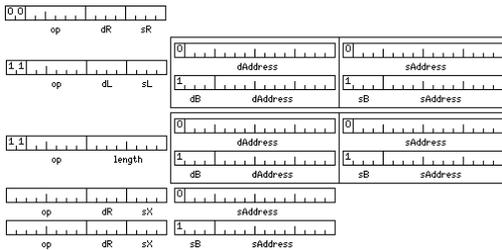
Only general registers 8 through 15 could be used as base registers. When the first bit of a 16-bit address field in an instruction was a zero, then the remaining 15 bits were used as an address, without the need to add the contents of a base register to it. Where it is shown for the memory to register instruction format, that format is simply divided into two formats, one for each case; it also applied to both address fields in the decimal and string instructions as well, and there boxes
