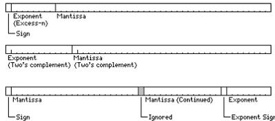
The format shown in the first line begins with a single sign bit, which is 0 if the number is positive, and 1 if the number is negative. Next is the exponent. If the exponent is eight bits long, as shown in the diagram, it is in excess-128 notation, so that the smallest exponent value, 00000000, stands for -128, and the largest exponent value, 11111111, stands for 127. Finally, we find the mantissa, which is an unsigned binary fraction.
