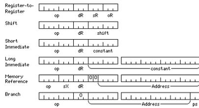
Addresses point to 64-bit words, and thus two additional packet select bits are required in branch instructions, where a unit of 16 bits is referred to as a packet.
