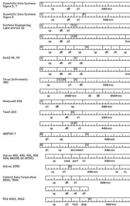
The first instruction format shown is the instruction format for the SDS Sigma series of computers, for which all instructions were 32 bits long.
