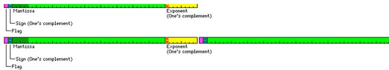
The Manchester ATLAS computer, notable for introducing virtual memory, used an 8-bit sign-magnitude exponent followed by a 40-bit sign-magnitude mantissa. The exponent was a power of eight. A power-of-eight exponent was also used on the Burroughs 5500; thus, a claim I once read that a power-of-eight exponent did not, in practice, lead to the type of problems encountered with the power-of-sixteen exponent on the IBM System/360 could have had practical experience behind it.
